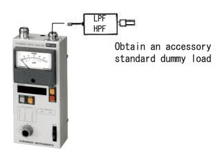
Connect and measure  $50\,\Omega$  dummy loading of the attachment on the load side. The range etc, of the operation frequency can be measured for the frequency characteristic and the tuner in case of the filter.
