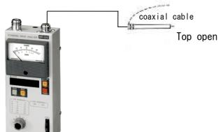
Whip antenna for handy transceiver when using it to test
