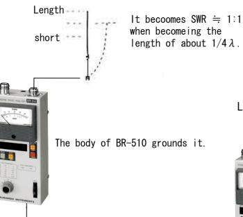
Ground the body of applying Counterpoiz of  $1/4 \lambda$  to the body or this machine when the electric wave length in long.
