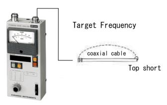
How long is the wave of coaxial cable? Measurement is impedance. Measurement of  $1/2\,\lambda$  or n( $1/2\,\lambda$ ), coaxial cable is shorting top side. How long is coaxial cable? Measurement is Impedance zero or minimum data. (How long is transmitter to antenna?)
